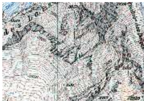
Figure 19: Rock representation with ridges and contour lines. Part of a test map of Dent du Midi, Swiss Federal Office of Topography, 1938.
