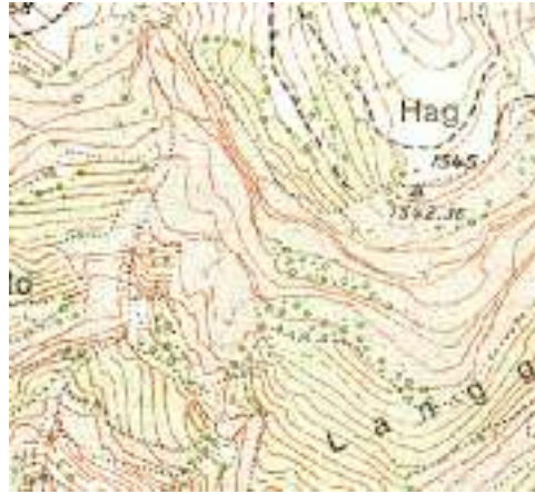
Figure 22: A test of a very simple rock representation (“Fels in reiner Kurvendarstellung”). Original scale 1:10 000, 1922. Source: [Kraiszl, 1930].
