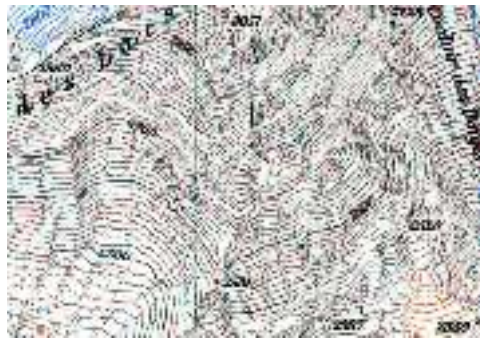
Figure 14: Rock representation with contour lines only. Part of a test map of Dent du Midi, Swiss Federal Office of Topography, 1937.
