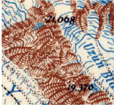
Figure 6: Fill hachures style, as drawn by Yates. Source: Karakoram Himalaya map of the Royal Geographical Society, 1939.
