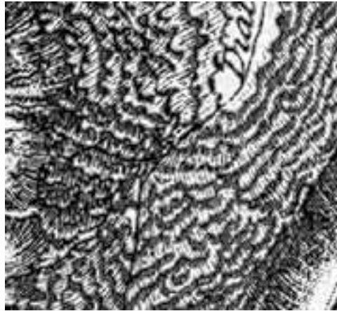
Figure 4: Rock hachures as drawn in the early 19th century by Roverea and Grunder. Source: [Kraiszl, 1930]
