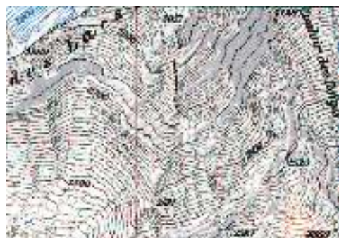
Figure 13: Rock representation with few contour lines and colour tones. A test map of Dent du Midi, Swiss Federal Office of Topography, 1938.
