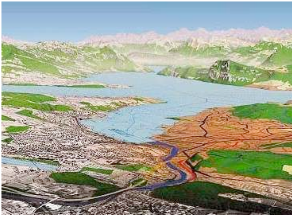
Fig. 3: Raster and vector maps, orthophotos and satellite imagery can be combined and draped on top a digital terrain model to produce spectacular views.
