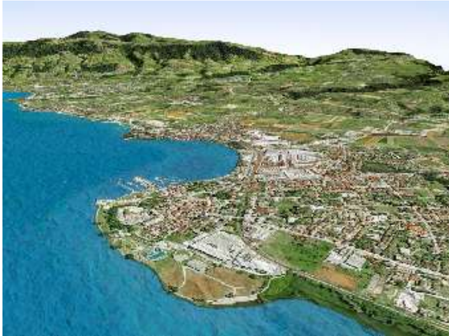
Figure 2: Perspective view of the Lake of Constance, Switzerland created by draping an orthophoto onto a digital terrain model (Dobler 2001). (DTM: © Federal Office of Topography, Wabern; orthophoto: © Swissphoto)
