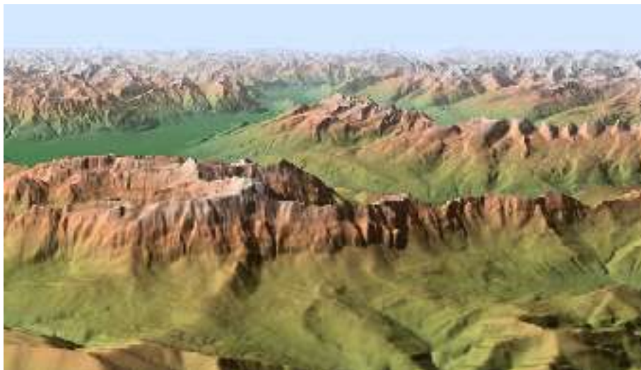
Figure 5: A panorama of the Säntis mountains, Switzerland, created from coloured hypsometric tints applied to a DTM (Atlas of Switzerland 2000).
