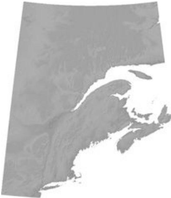
Figure 5. GTOPO30 data, cropped at 40° to 55° North by 60° to 78° West and reprojected in UTM.
