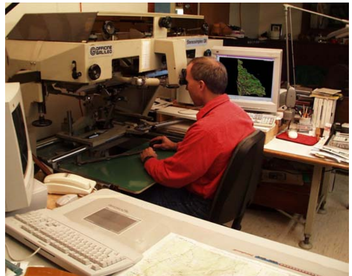
Figure 1 - Tracing maps: an unconventional use for a stereoplottor
