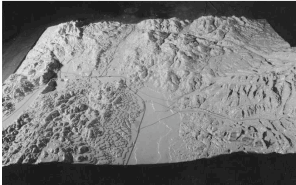
Figure 14. A physical model of the Deer Lodge and Silver Bow Valleys near Butte, MT. Todd Trigsted created this model for the Montana Water Company by stacking cardboard cutouts based on topographic contours. (Courtesy of Todd Trigsted).
