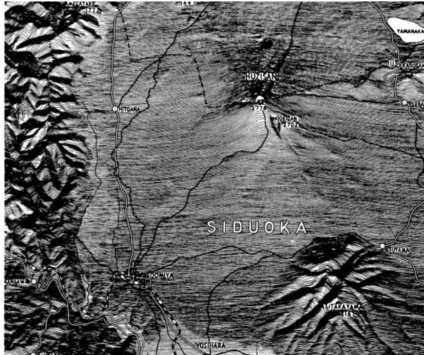
Figure 2. An inclined contour map of a portion of Mt. Fuji, Japan. The inclined plane used to define the traces had a strike of E-W and a dip of 45^\circ to the south. (Reprinted from Tanaka, 1932 (Plate 2 on page 212) with permission from the Geographical Journal)
