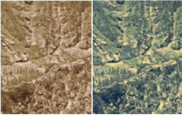
Figure 4: *Color Transfer to Grayscale Orthoimage*. Fully automatic statistical method is used to transfer color from a sample source image to a grayscale target image by making statistical color distribution in the target image equal to the distribution in the source image. Different source images were applied to the same grayscale target image.
