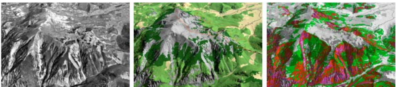
Figure 4. Visualisation of Mt. Schneeberg near Vienna, Austria: Photorealistic visualisation using orthophoto draped over landscape (top). Symbolised visualisation of land cover and touristic infrastructure (centre). Overlay with slope and aspect information (bottom). Source: Karel Kriz, University of Vienna
