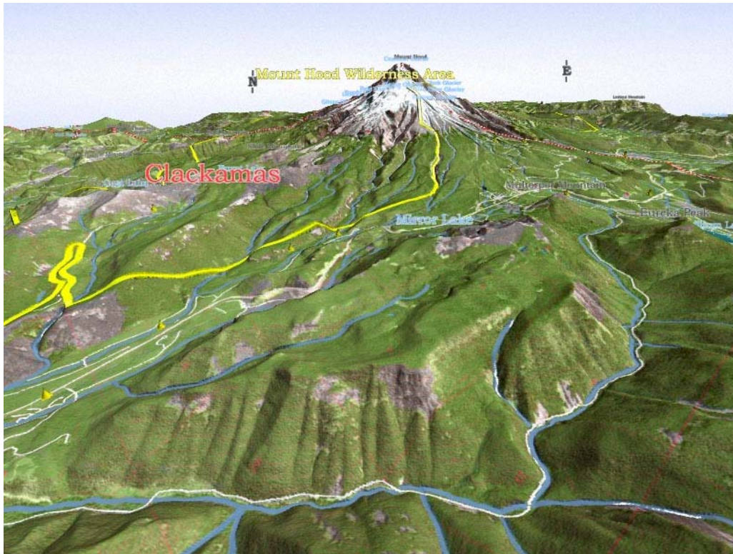
Figure 6. 3D-visualisation of Mt. Hood/Oregon/USA: DEM overlaid with topographic map elements, orthophoto, vector linework and labels. See [wwwHood].
