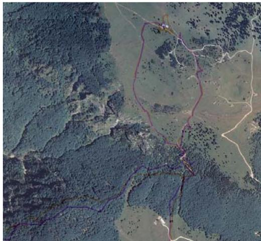
**Figure 2:** two GPS receivers' survey vs. orthophoto
