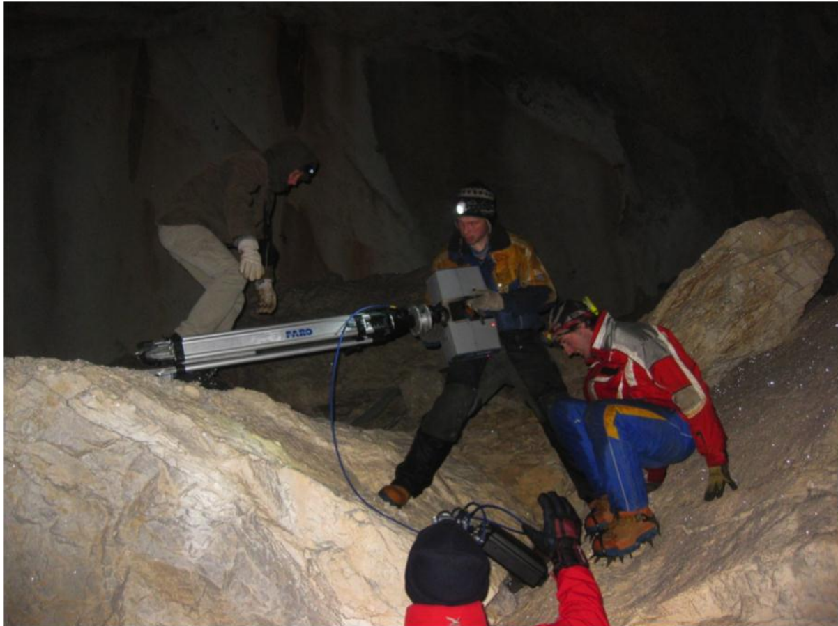
Figure 5: Demanding work to mount the TLS at the required positions.
