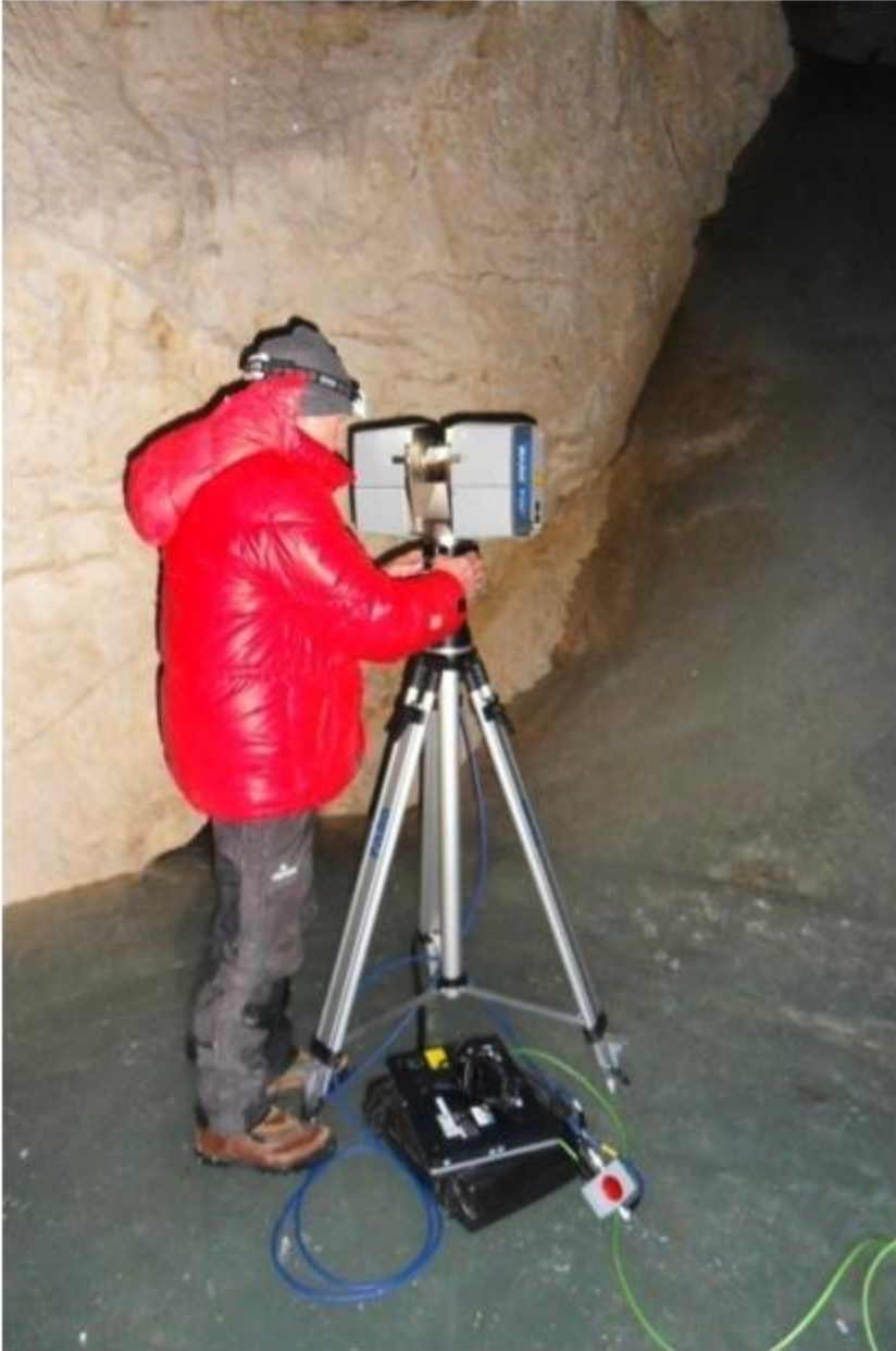
Figure 3: The author operating the FARO Photon 20/120 on the cave ice surface.
