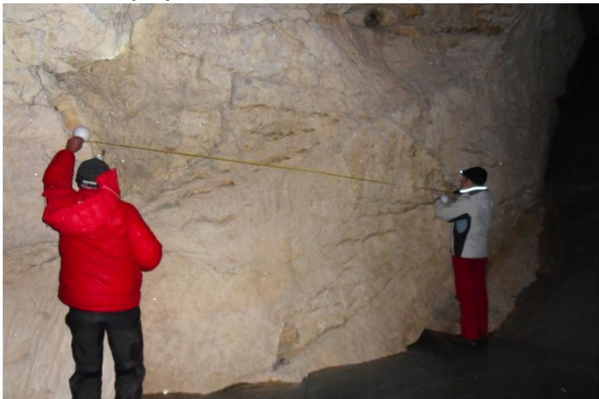
Figure 2: “Classical” tape measure surveying of the styrofoam reference globes.
