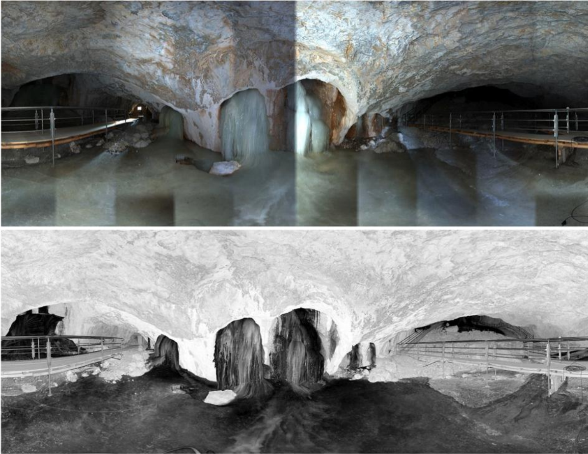
Figure 6: Depiction of both a TLS scan using FARO Photon 20/120 in the outer Eisriesenwelt, taken 7 April 2010. Top: Point cloud. Bottom: Synchronously taken digital photograph for texture draping.
