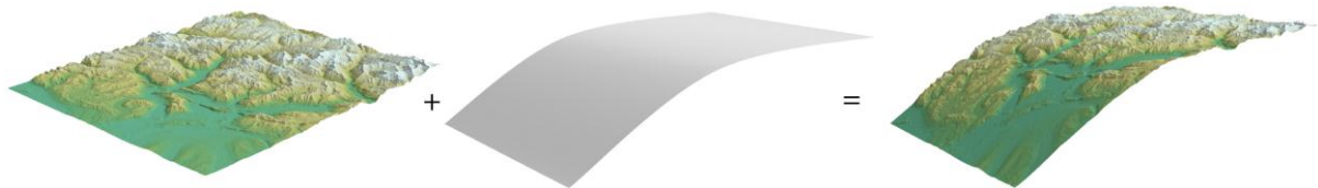
Figure 3 Concept of the global progressive bending method: altitudes in the undeformed elevation model (left) are combined with a bent terrain base (middle) into a bent elevation model (right)
