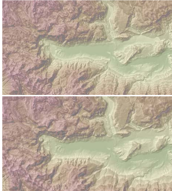
Figure 13: Combination of hill shading and enhancement of the ridges with peaks using bipolar differentiation (all three in light and dark casts) with interval of bipolar differentiation light contrasts of 100 m (left) and 250 m (right). The fourth method used here is hypsometry using different colours.
