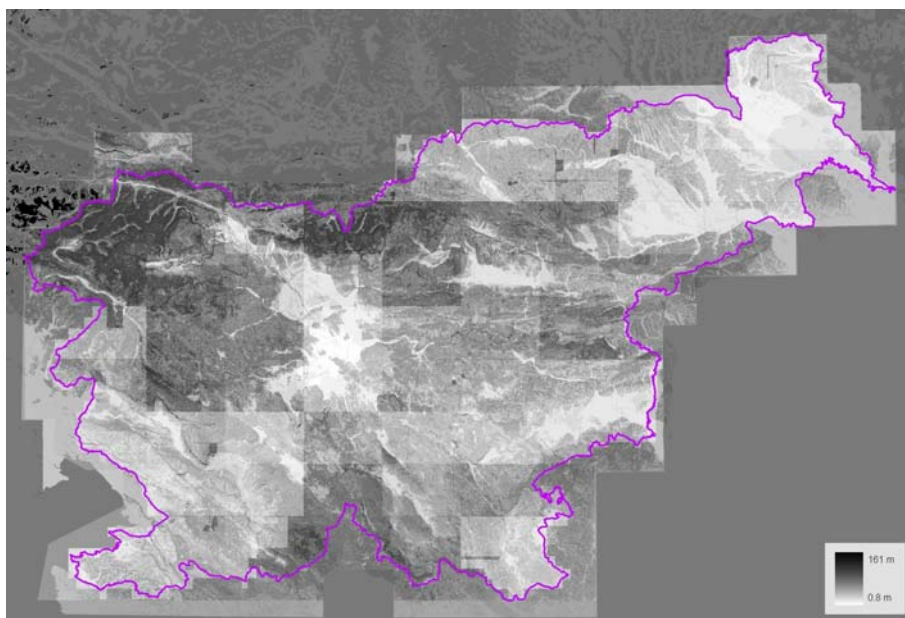
Figure 6: Potential random error for DEM of Slovenia in grid 12.5 x 12.5 m regarding different data sources used
