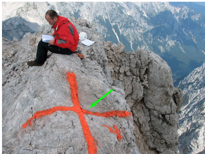
Figure 4: An example of a control point stabilised with a screw (green arrow) and marked with a non-permanent colour made in 2005 for the filming in the scale of 1:5000 (photograph taken by Blaž Barborič and Matija Klanjšček).
