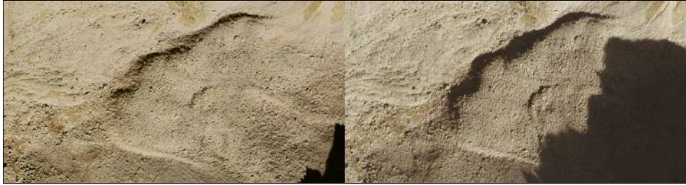
Fig. 12 Multi-temporal (pseudo) stereogram of Leibnitzkopf rock glacier. Left stereopartner (orthophoto, 18 September 2002) taken from Google Maps. Right stereopartner (orthophoto, 21 September 2006) taken from Microsoft Bing Maps. Parallaxes introduced by motion can be perceived stereoscopically as “hills” and “valleys” depending on the direction of motion. The main flow/creep direction has to be parallel to the eye base of the observer
