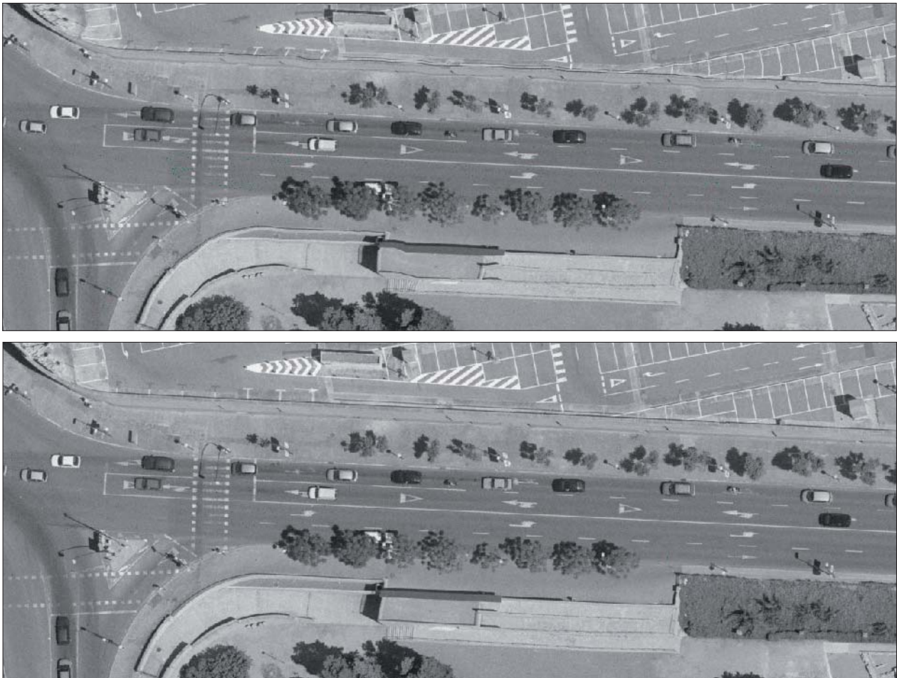
Fig. 7: The upper image shows a detail of an orthophoto rectified using a DSM obtained from LIDAR data. The lower image shows the result using a DSM obtained by stereoplotting.
