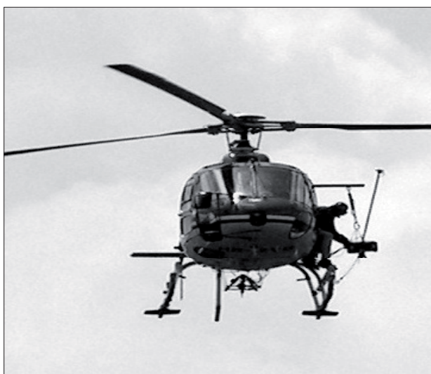
Fig. 2: Vertical (nadir) and oblique configuration of the system
