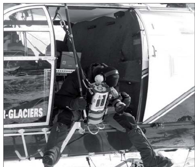
Fig. 3: Components of the Helimap System. A camera, GPS receiver, Inertial Unit and laser scanner.
